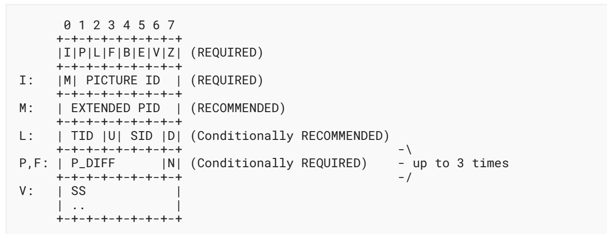
Figure 2: Flexible Mode Format for VP9 Payload Descriptor
